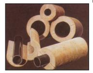
Mandrel wound and concentrically formed form fitting pipe sections, precisely made to fit standard pipe diameters offer uniform maximum resistance to passage of heat along and around the entire 360° of the pipe axis. Superior density of this product enhances compression resistance in service. These sections are easy to fit and hence afford speedy application at site.
