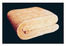
ROCKLOYD, like all scientifically processed fibrous insulants is composed of fibres which are laid in the optimum configuration to offer maximum resistance to heat flow. To retain these exceptional properties up to the point of enduse, fibres are interlocked by lightly bonding them together using a thermosetting binder. Subsequently, matts are factory stitched to specified wire mesh
